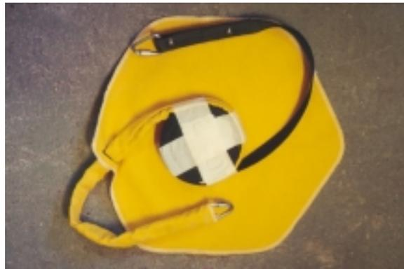
The drogue parachute is an R3C by Rocketman, with extra heavy shroud lines. It will provide a full-loaded descent rate of about 70 fps. The main parachute is an R14C Rocketman with nomex bag deployment system. When both parachutes are deployed, they will provide a fully loaded descent rate of about 15 fps. The nomex bag is attached by bridle to the peak of the main parachute canopy.
