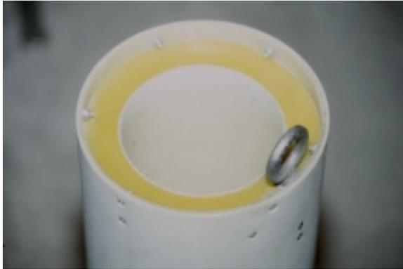
This is the forward end of the fin can showing the G10 coupler and centering ring. Note the 12 bolts holding the fore and aft retaining rings, which provide a sturdy attachment for the centering ring.
