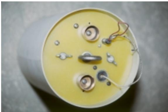
A close up of the aft end of the electronics bay shows another recovery beeper, which is activated on drogue deployment. A clear plastic cap on a string protects the beeper from ejection gasses.
