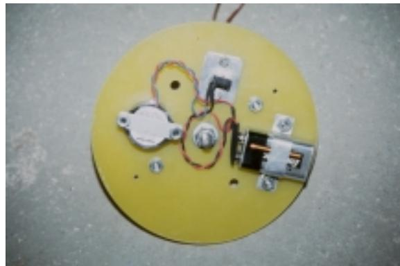
Details of the back of the electronics bay bulkhead show the mounting and wiring of the recovery beeper. The simple circuit is activated when a headphone plug is pulled out of it's jack on ejection.
