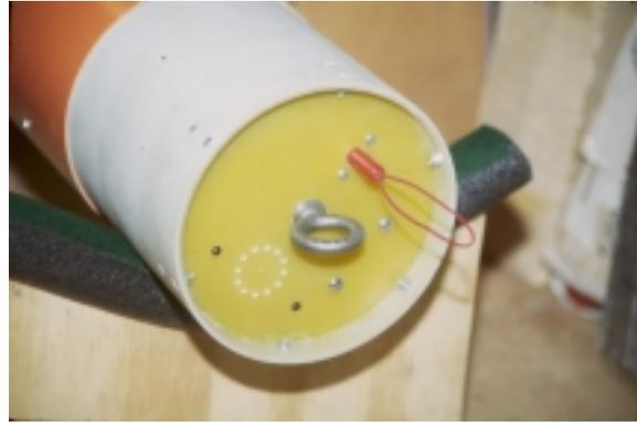
The payload bulkhead is attached to the coupler in the same fashion, with 12 bolts holding fore and aft retaining rings. The coupler is attached to the payload airframe by the standard 8-32 bolt pattern.
