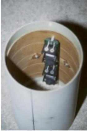
The main electronic control for recovery is a Black Sky Research AltAcc, which uses an accelerometer for determining drogue deployment, and a pressure transducer to determine the proper altitude for main parachute deployment. Backup electronic control is via second AltAcc or a BSR timer. The timer will be programmed with deployment times determined by computer simulation, and will control its own separate ejection charges.
