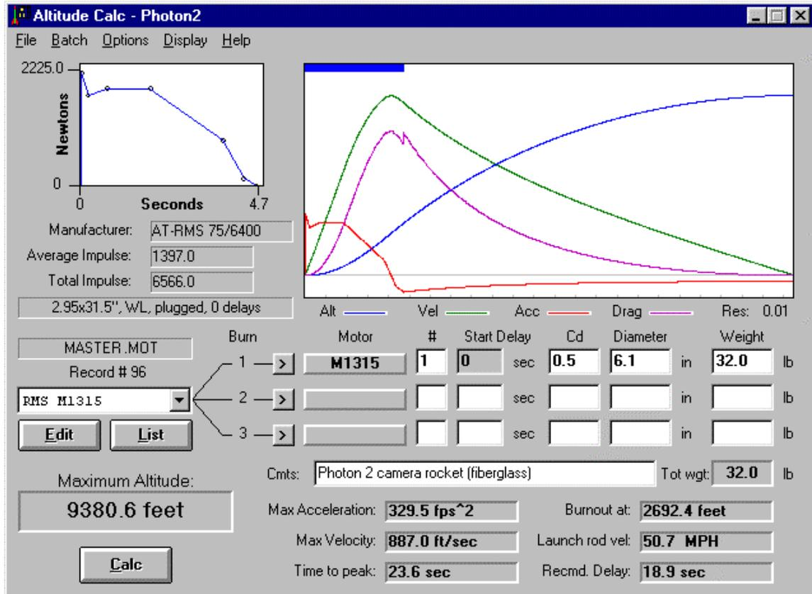
Thrust Curve: Motor data for the Photon Alticalc simulation was obtained from Aerotech.
